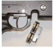
To load pellets into the magazine, remove as above. Load pellets nose first into the recessed side of the 8 shot drum magazine - (the flat side). Push the pellet nose through the retaining rubber O-ring until its skirt lies flush or below the bottom of the magazines rear face.
