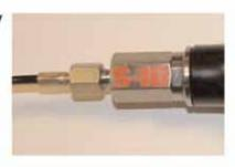
5) When charging is complete, "bleed" off the excess air from the hose using the hoses's bleed screw. Then unscrew the bottle from the charging adaptor.
